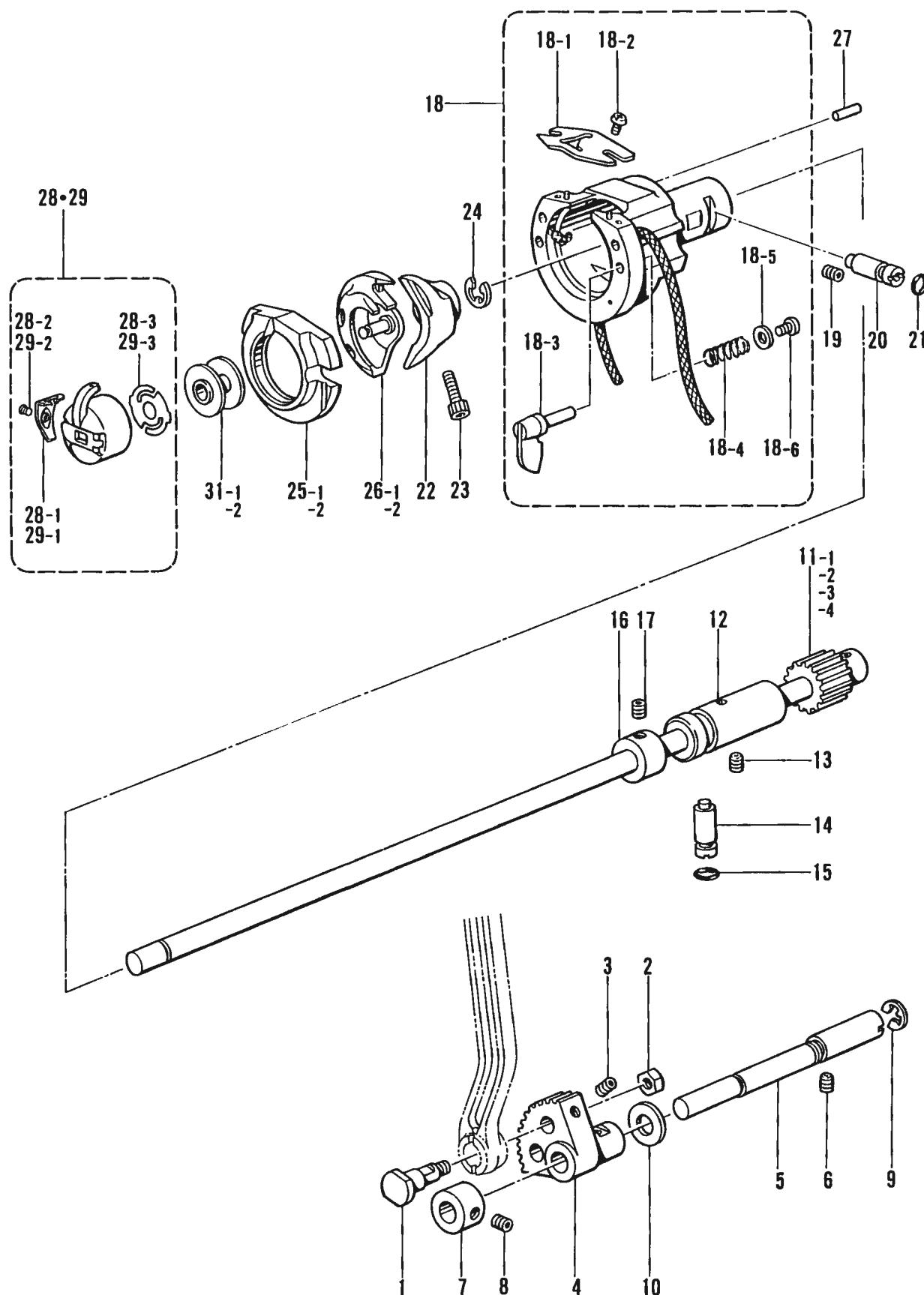
F. 下軸関係 / Lower shaft mechanism / Untere Welle /
