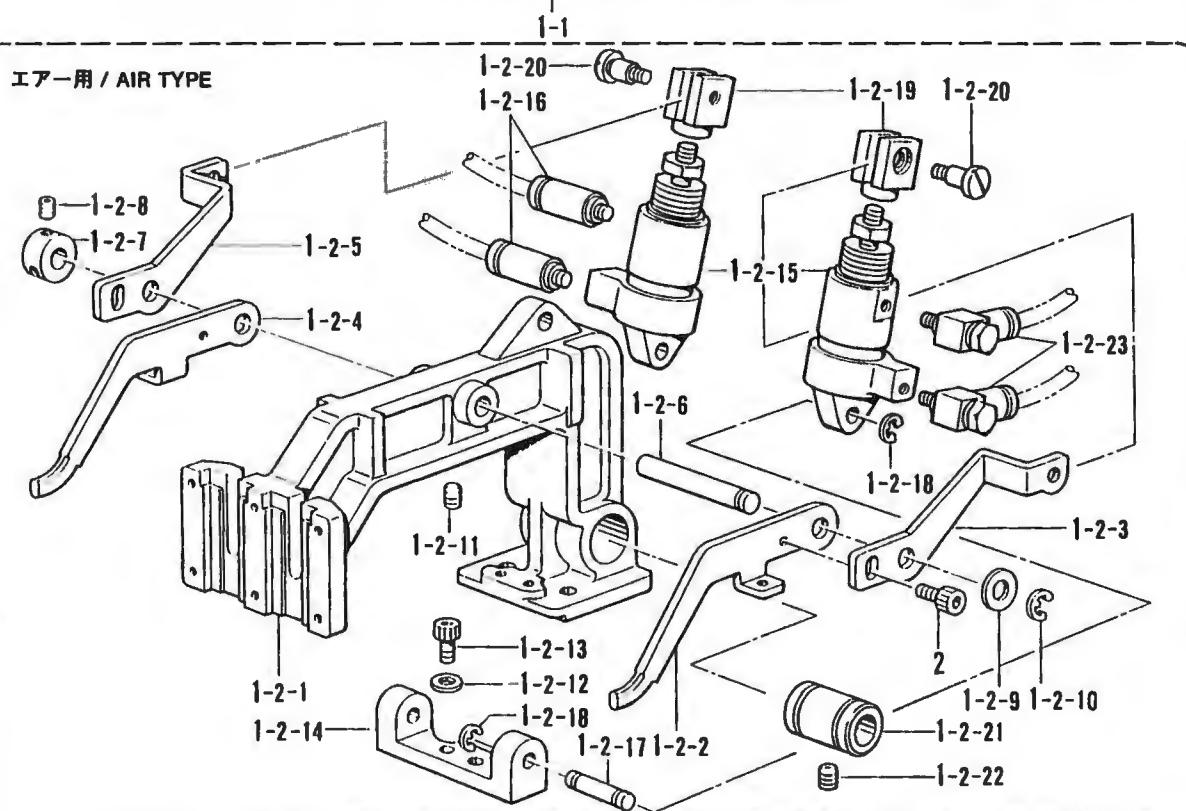
C. 送り関係 / Feed mechanism / Transportvorrichtung /
